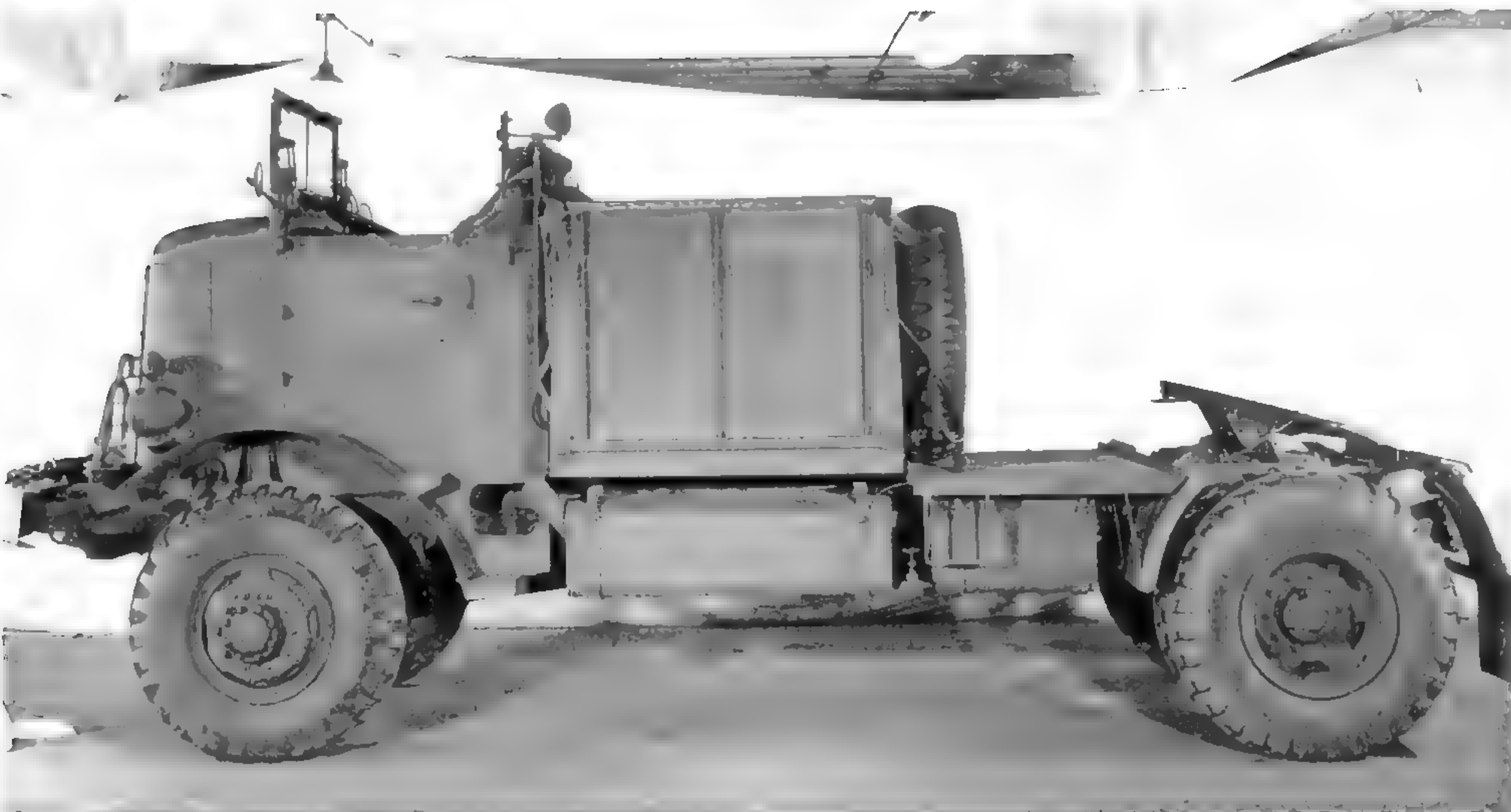
The doors on either side of the large toolbox behind the U8144-T cab opened by swinging down. A spotlight was mounted on the rear of the driver's side of the cab to aid in night work. (U.S. Army photo)
